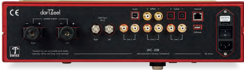
ABOVE: Four single-ended line inputs are joined by pairs of coaxial and optical S/PDIF digital ins, asynchronous USB-B and network audio ports. Clamp-down speaker binding posts are best suited to cable or spade connectors
